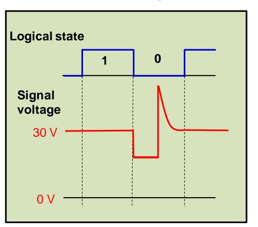
A Bit in KNX TP: Logic "0"  $\rightarrow$  current drawn Logic "1"  $\rightarrow$  no current drawn
