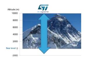
Average Sea level pressure = 1013.25 mbar (varies with weather) Pressure decrease when altitude increases Monitoring under / over pressure
