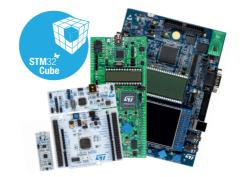
A full set of evaluation boards enables flexible prototyping as well as full STM32L4 evaluation. Commercial part numbers: NUCLEO-L432KC (32 pins); NUCLEO-L476RG (64 pins); STM32L476G-DISCO; STM32L476G-EVAL
