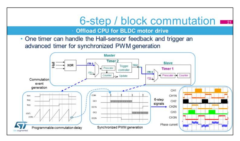
This slide shows how the 6-step drive (also called block commutation) is managed with the STM32 timer.
