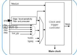
A given timer can simultaneously operate in slave and master modes in a cascaded configuration
