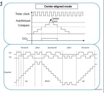
Some of the STM32 timers feature up/down counting modes: the advanced control timers 1 and 8 and the general-purpose timers 2, 3, 4 and 5.
