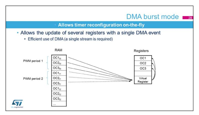
The timer includes a DMA burst mode to have multiple registers re-programmed with a single DMA stream. This allows the modification of several run-time parameters simultaneously (for instance duty cycle and frequency of several channels) or dynamically change the timer configuration by writing the configuration registers.
